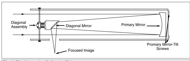
Fig. 4: The Newtonian Reflecting Telescope.
